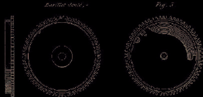
Louis Moinet study of a toothed barrel leading to his discovery of a mainspring improving the rating of the watch
